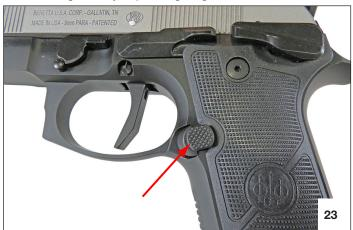
Press and hold the disassembly lever release button.
