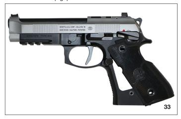
Install the lock washers and grip screws with a 2 mm allen wrench by turning them clockwise. Tighten the grip screws to a torque of 10 lb·in.
