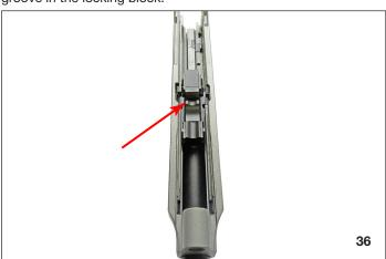
Make sure the barrel locking assembly is in rear-most position. If necessary, push the barrel locking assembly to the rear using the open area at the slide.
