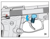
Pull the slide-barrel assembly with locking block, recoil spring and spring guide forwards
