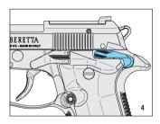
Pull back the slide and release it. The slide will automatically pick up a cartridge from the top of the magazine and feed it into the chamber.
