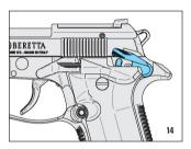
warning: Always ensure that the safety is fully engaged until ready to fire. A safety is fully engaged only when the safety can move no further into the safe position. A safety which is not fully engaged will not prevent weapon discharge.
