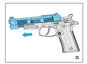
Slightly press recoil spring and spring guide and lift it to re-
