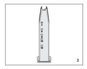
Repeat process until magazine is fully loaded. Holes on the back of the magazine allow for visual counting of cartridges.
