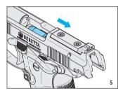
A WARNING: THE PISTOL IS NOW CHAMBER LOADED, COCKED, THUMB SAFETY DISENGAGED AND READY TO FIRE BY PULLING THE TRIGGER.
