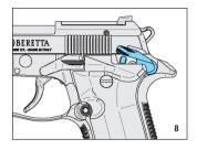
Keep the pistol pointed in a safe direction and remove the magazine from the pistol.
