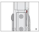
The tab is located on the right side of the pistol's slide, near the chamber, and can be both seen and felt, allowing the user to check the chamber at night by feel or during the day by checking for the increased protrusion of the red tab.
