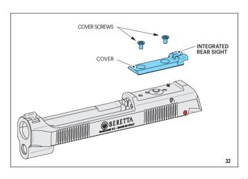
detached it may fly back and strike the shooter or bystander and cause injury. Observe the condition of the mounting screws after firing. If the mounting screws show signs of loosening DO NOT fire the gunagain until you have re-tightened the screws. The original screws come with a drop of glue applied; if it could not be enough the use of Loctite® is recommended.
