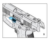
To fire again, remove the empty magazine and insert a loaded one.
