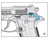
A WARNING: Always ensure that the safety is fully engaged until ready to fire. A safety is fully engaged only when the safety can move no further into the safe position. A safety which is not fully en-
