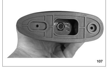
3. Align the recoil pad to the stock and secure with two phillips screws.
