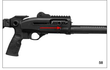
3. Press the head of the breech bolt until the groove on its neck is aligned with the edge of the bolt body. with the groove aligned pull outward on the bolt handle to remove it from the bolt
