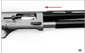
7. Slide the forend into place over the gas cylinder/the valve assembly and magazine tube, checking for the correct centering on the receiver face. The forend is in the correct position when it is fully against the receiver.
