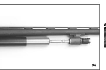
6. Push the barrel all the way into the receiver until it stops.
