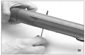
4. Keeping the breech bolt release button pushed all the way down, remove the trigger pack from the receiver using the trigger guard as a lever, first in the direction of the barrel and then outward.
