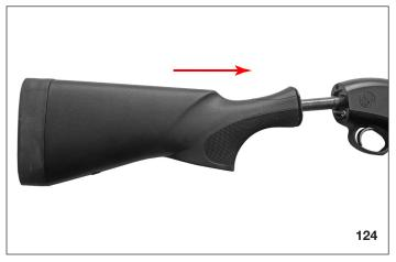
Using the 13-mm socket wrench, install the retaining nut and washer to the stock bolt. Tighten to a torque 60 lb-in (7 N•m). The use of a proper torque wrench is recommended.
