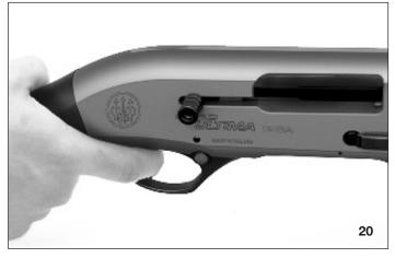
12. Engage the safety (red ring not visible), and if necessary, reload the shotgun according to the previous instructions.
