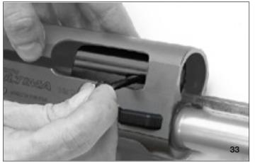
4. Over a flat surface, with the ejection port pointed upwards, slide the connecting rod with sleeve forward off the magazine tube shaft to extract the breech bolt assembly from the receiver.
