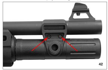
5. Unscrew forend cap in a counterclockwise direction.
