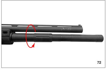
5. Remove the magazine spring from the magazine tube.
