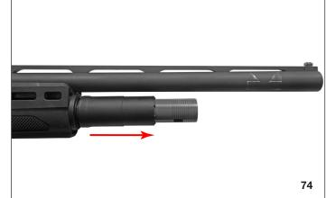
7. Holding the shotgun by the barrel, pull the forend straight out toward the muzzle.
