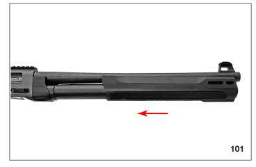
4. Verify proper orientation of the magazine cap sleeve as noted during the removal. Slide magazine cap sleeve onto the magazine tube.
