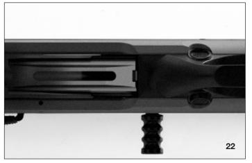
2. Pull back the breech bolt to extract and expel the live cartridge from the chamber.
