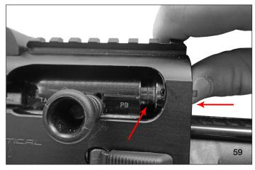
4. Over a flat surface, with the ejection port pointed upwards, slide the connecting rod with sleeve, recoil spring, and spring holder forward off the magazine tube shaft to extract the breech bolt assembly from the receiver
