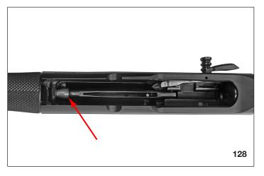
4. Once properly aligned, Insert the cocking handle into the breech bolt.
