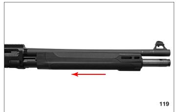
6. Verify proper orientation of the magazine cap sleeve as noted during the removal. Slide magazine cap sleeve onto the magazine tube.
