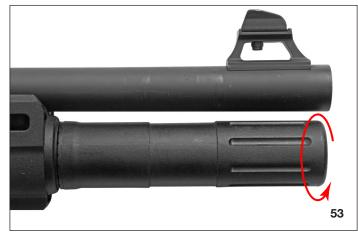
5. Remove the magazine cap sleeve from the magazine tube.
