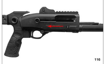
3. Insert the barrel into the receiver, ensuring that the magazine tube shaft enters the piston hole as well as that of the gas cylinder and the valve assembly.
