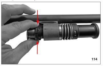
1. Press the the carrier stop push button all the way down.
