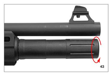
6. Remove the magazine cap sleeve from the magazine tube.
