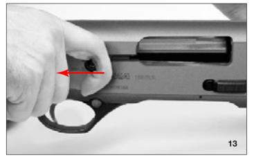
3. Engage the manual safety by pressing the safety button to hide the red ring.
