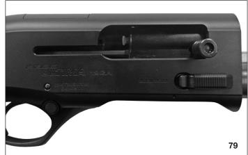
5. Over a flat surface, with the ejection port pointed upwards, slide the connecting rod with sleeve forward off the magazine tube shaft to extract the breech bolt assembly from the receiver.
