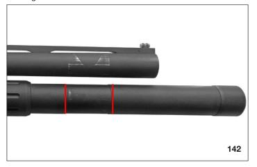
12. Tighten the two hex screws to 18 in. lb. Do not over tighten the two hex screws, see warning below.
