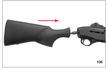
Using the 13-mm socket wrench, install the retaining nut to the stock bolt. Tighten to a torque 60 lb-in (7 N•m). The use of a proper torque wrench is recommended.
