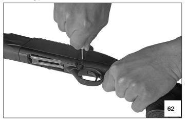
3. Remove the trigger pack from the receiver using the trigger guard as a lever, first in the direction of the barrel and then outward.
