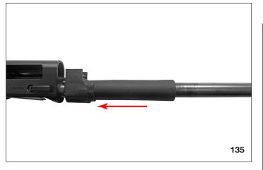
6. Insert the barrel into the receiver, ensuring that the magazine tube shaft enters the piston hole as well as that of the gas cylinder and the valve assembly.
