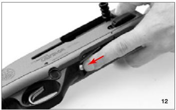
2. Use the cocking handle to retract the breech bolt until it snaps into the open position.
