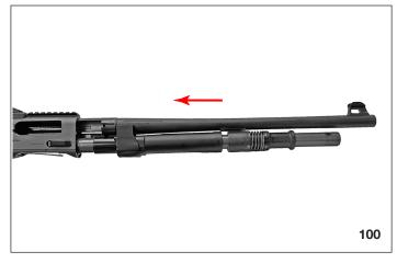
3. Slide the forend into place over the gas cylinder/the valve assembly and magazine tube checking for the correct centering on the receiver face.
