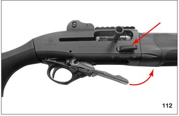
3. Insert the trigger guard retaining pin only when the hole of the trigger guard is centered on the receiver.
