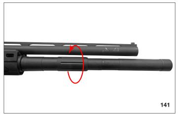
11. Align the barrel clamp inside the stepped down area of the magazine extension.
