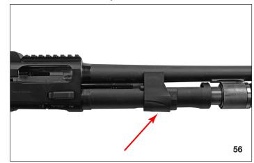
8. While holding the piston inside the gas cylinder of the barrel, pull the barrel out of the stock-receiver assembly.
