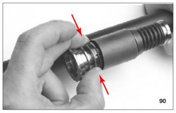
3. Check that the carrier stop push button is pressed all the way down. If it is not, push it all the way down.
