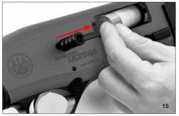
5. Keeping your hands away from the ejection port, press the breech bolt release button and guide the breech bolt to the locked position.
