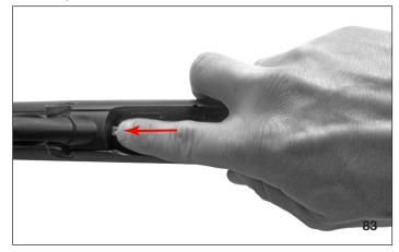
3. Using a pin punch or an awl, Remove the trigger guard retaining pin.
