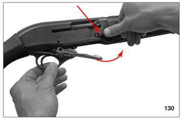
3. Insert the trigger guard retaining pin only when the hole of the trigger guard is centered on the receiver.
