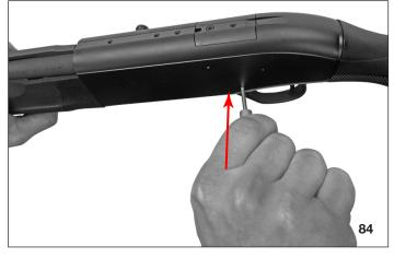
4. Keeping the breech bolt release button pushed all the way down, remove the trigger pack from the receiver using the trigger guard as a lever, first in the direction of the barrel and then outward.
