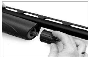
4. Holding the shotgun by the barrel, pull the forend straight out toward the muzzle.
