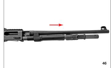
8. Remove the barrel assembly from the receiver.
