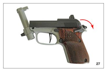
Retract the slide about 1/8 inch and lift the front of the slide over the barrel hinge.
