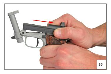
Press down on the front of the slide until it clicks. The click indicates the engagement between the recoil spring and the slide cutouts.
