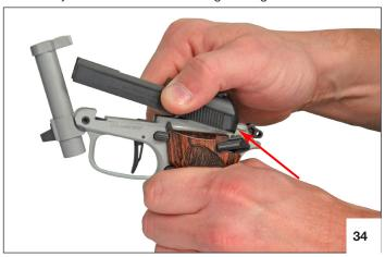
Pull the slide rails back over the frame's guide lugs; simultaneously, lower the front end of the slide down to gently rest on the frame (top of the recoil spring levers),
