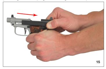
Quickly release the slide. The slide will automatically close, chambering the first cartridge from the magazine. The hammer is fully-cocked. The pistol is ready to fire.
