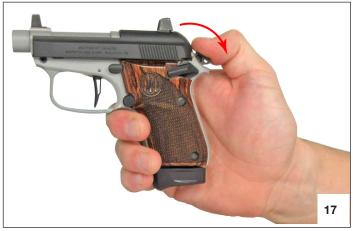
Gradually release the thumb pressure, allowing the hammer to move forward a short distance to solid hammer/ sear engagement.
