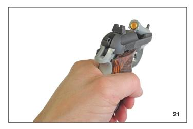
Depress the magazine release catch and remove the magazine from the pistol.
