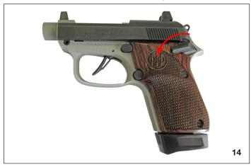
Grasp the slide serration with thumb and index finger (keep finger outside the trigger guard), retract the slide until it stops (activating the recoil springs and cocking the hammer).
