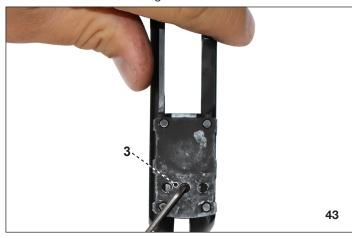
Slide the rear sight into the dovetail slot. Using a 1.3mm allen wrench, secure the rear sight in position with the set screw (4).
