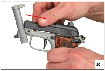
Once the sharp click is heard, pull the slide forward until it clears the frame guide lugs.
