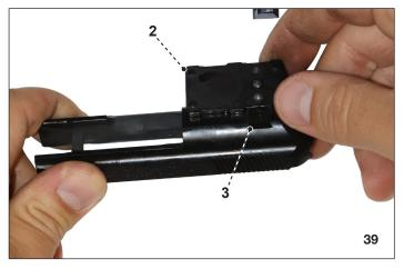
Using a 2mm allen key, install and tighten the optic plate set screw (4) into the threaded center hole, securing the optic plate to the slide.
