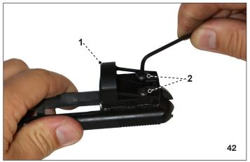
Using a 2mm allen wrench, unscrew the optic plate set screw (3. and slide it out of the rear sight dovetail slot.
