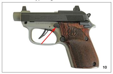
Insert a cartridge into the chamber, and push the barrel down. A sharp click indicates barrel lever engagement.
