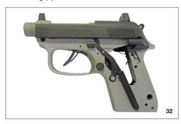
Install the grip screws with a flathead screwdriver by turning them clockwise. Tighten the grip screws to a torque of 10 lb·in.
