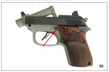
Swing the barrel forward over its hinge until it reaches a solid stop.
