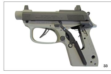
Install the grip screws with a flathead screwdriver by turning them clockwise. Tighten the grip screws to a torque of 10 lb-in.
