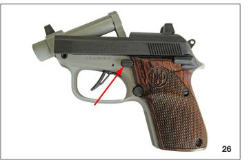
3. Swing the barrel forward over its hinge until it reaches a solid stop.
