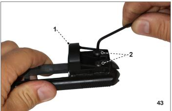
2. Using a 2mm allen wrench, unscrew the optic plate set screw (3. and slide it out of the rear sight dovetail slot.
