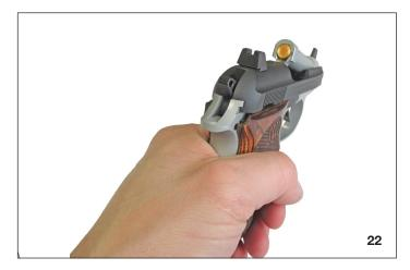
2. Depress the magazine release catch and remove the magazine from the pistol.
