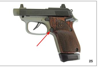
2. Press the barrel latch to release the barrel.
