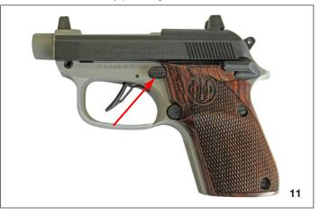
3. Insert a cartridge into the chamber, and push the barrel down. A sharp click indicates barrel lever engagement.
