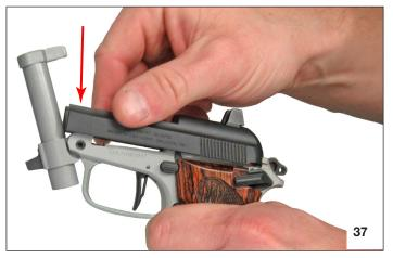
**NOTE:** Visually inspect that the underside of the slide is resting flat against the frame's sliding surface (slide and frame are parallel).
