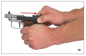
4. Quickly release the slide. The slide will automatically close, chambering the first cartridge from the magazine. The hammer is fully-cocked. The pistol is ready to fire.
