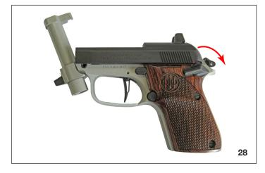
4. Retract the slide about 1/8 inch and lift the front of the slide over the barrel hinge.
