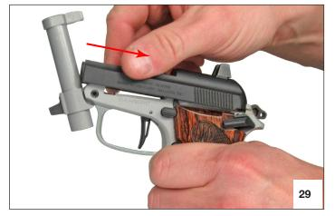
5. Once the sharp click is heard, pull the slide forward until it clears the frame guide lugs.
