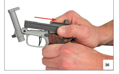
4. Press down on the front of the slide until it clicks. The click indicates the engagement between the recoil spring and the slide cutouts.
