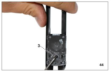
Slide the rear sight into the dovetail slot. Using a 1.3mm allen wrench, secure the rear sight in position with the set screw (4).
