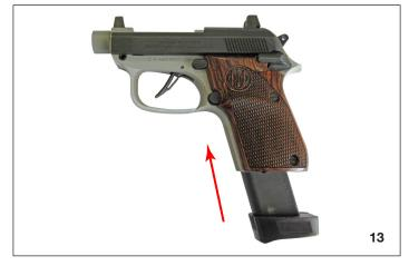
6. The pistol is now chambered and magazine loaded and ready to fire. Remember-when the hammer is fully-lowered to rest against the slide, the pistol can be fired by double action trigger pull (direct trigger pull-no manual hammer cocking).
