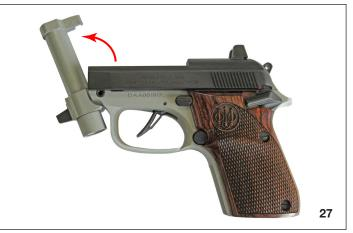
With the safety disengaged "OFF" (red dot showing) fully-cock the hammer.
