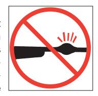
chamber(s) prior to loading to ensure that they are clean and free from obstructions. Firing with an obstruction in the barrel or chamber can rupture the barrel and injure you or others nearby. In the event you hear an unusual noise when shooting, stop firing immediately, engage the manual safety and unload the firearm. Make sure the chamber and barrel are free from any obstruction, like a bullet blocked inside the barrel due to defective or improper ammunition.
