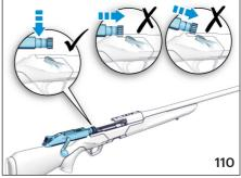
Refit the bolt carrier, making sure the guides are correctly coupled and that the bolt head is in the open position.
