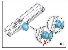
Refit the bolt head assembly into the carrier.
