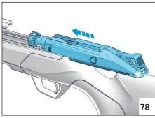
Push the carrier release button upward.
