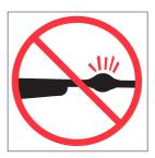
usual noise when shooting, stop firing immediately, engage the manual safety and unload the firearm. Make sure the chamber and barrel are free from any obstruction, such as a bullet blocked inside the barrel due to defective or improper ammunition.
