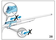
Press both release buttons to free the magazine.
