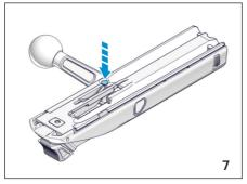
Take the bolt handle out of its seating (carrier side A).
