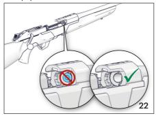
pull back the breech bolt to lock it into the open position and engage the safety before handing the firearm to another person. (see the "SAFETY" section on page 16);
