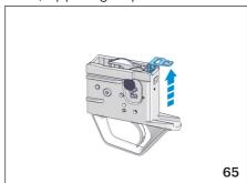
Before refitting the trigger housing, pull the trigger to release the hammer.
