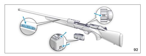
• Press both release buttons and remove the magazine.
