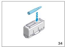
Insert the magazine into the loading gate with the tip of the cartridge facing forward.
