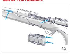
Insert the cartridges into the magazine (max. capacity: 5 cartridges).
