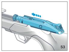
Push the carrier release button upwards.
