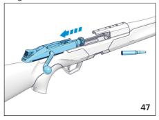
Empty any remaining cartridges from the magazine.
