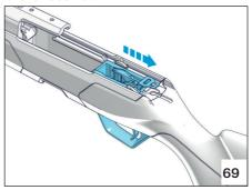
Press the safety and then the latch to lock the trigger group.
