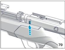
Slide the carrier out completely.
