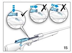
Proceed to fit the bolt carrier into the receiver: make sure the guides are correctly coupled.
