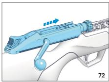
Make sure the guides are correctly coupled and that the bolt head is in the open position.
