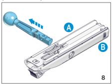
Insert the bolt handle fully into the seating (carried side B).
