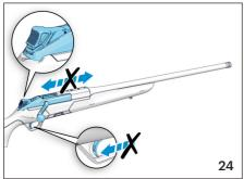
**3** Partial lock position: trigger locked, carrier free.
