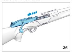
Move the carrier forward to chamber a cartridge.
