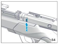
head screwdriver into the trigger group latch to lift the latch itself.
