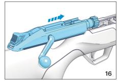
Check that the bolt head is in the open position.
